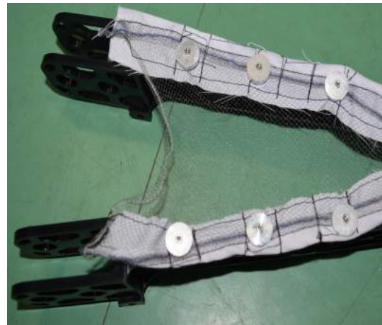
Figure 5.7: Mesh mounting using buttons on Two rib Fixture
