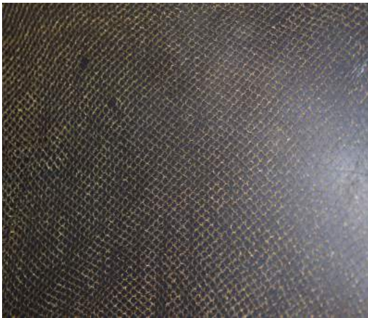
Figure 5.6: Gold plated molybdenum wire mesh
