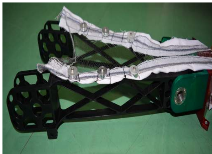
Figure 5.8: Mesh mounting provision using buttons on Two rib fixture
