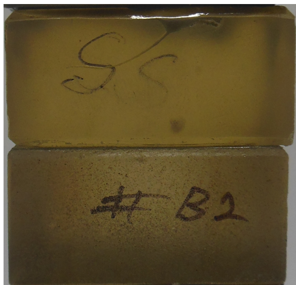
Figure 5.1: Zerodur pieces bonded with sodiyam silicate
