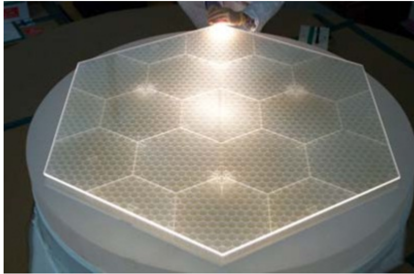
Figure 1.5: Telescope lightweighted mirror with honeycomb(Made by Kodak)[4]
