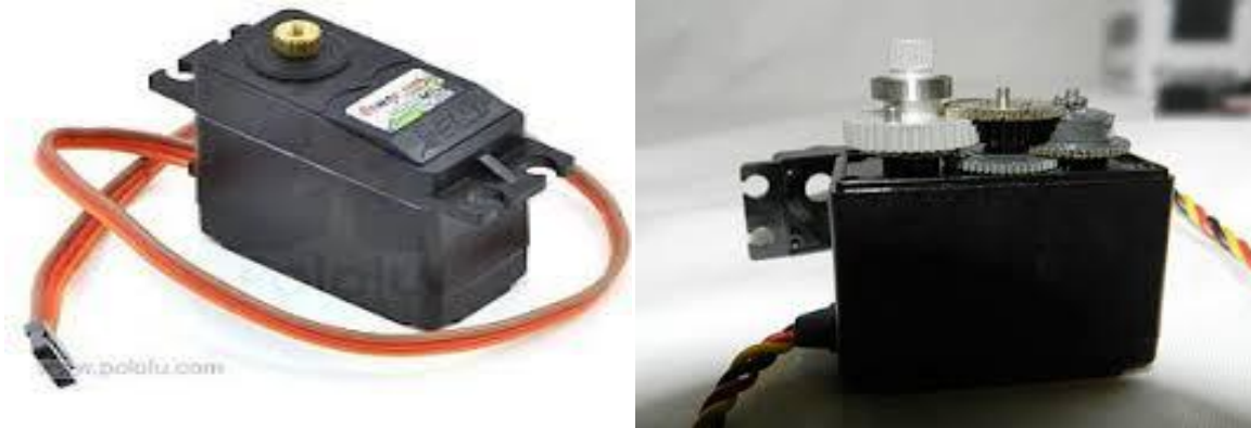
Fig. 5.9 Metal geared servo motor [22]
