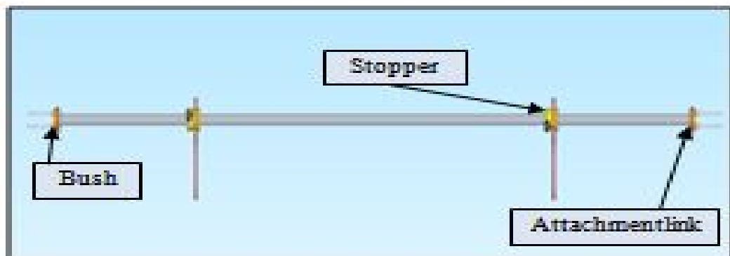
Figure 3.23: Front view of Hook/Gripper assembly
