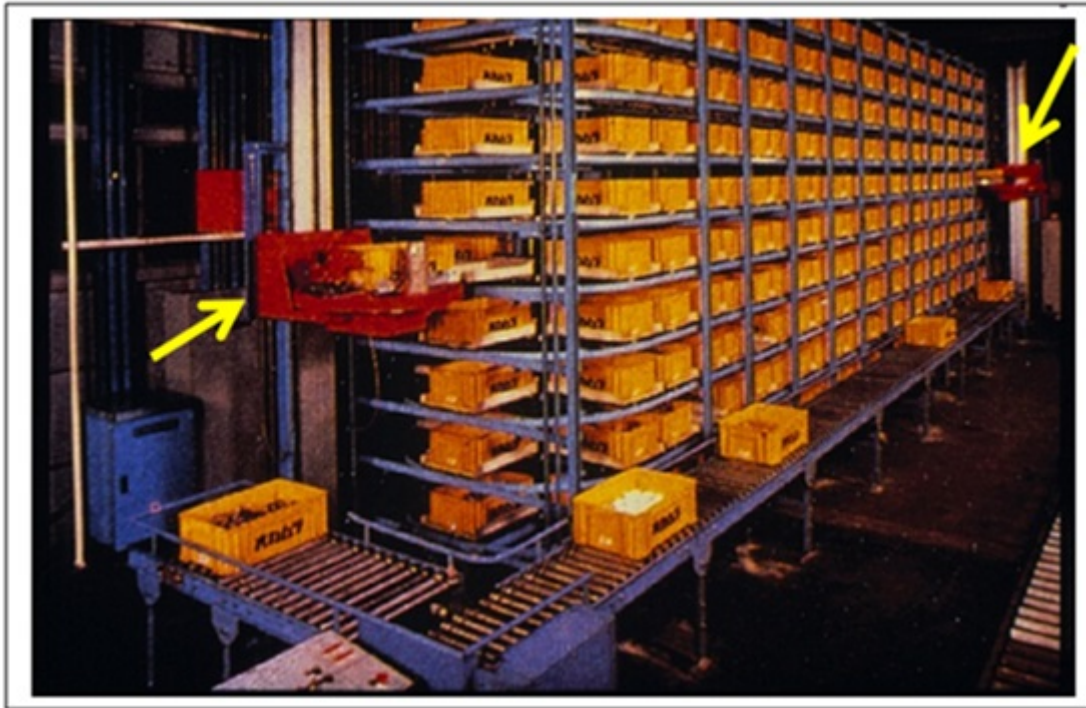
Figure 1.4: Independent Rotating Rack Storage system
