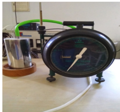
Figure 3.6: Gas flow meter
