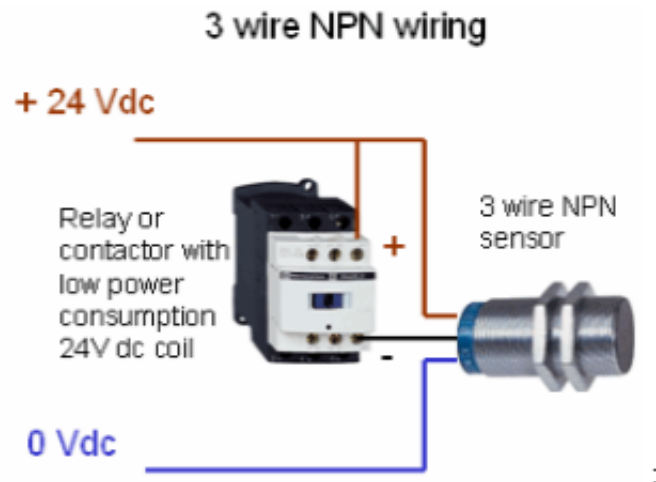
Figure 4.7: Proximity Sensor
