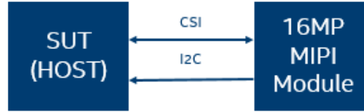
Figure 5.5: MIPI Camera Module Interface with Host
