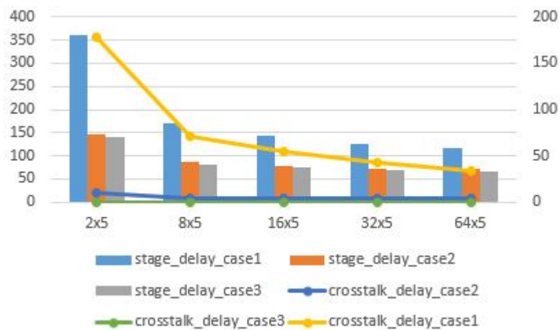
Figure 4.3.5: Graph of stagedelay and crosstalk delay versus different sizes for different cases having length of 250 micron for metal m3
