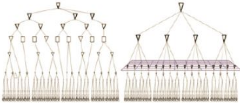
Figure 2.1.1: Set of sinks addressed by each of the two clock distribution methods[4]
