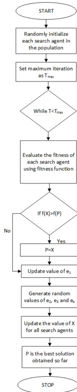
Figure 4.5: Flowchart of Sine Cosine Algorithm
