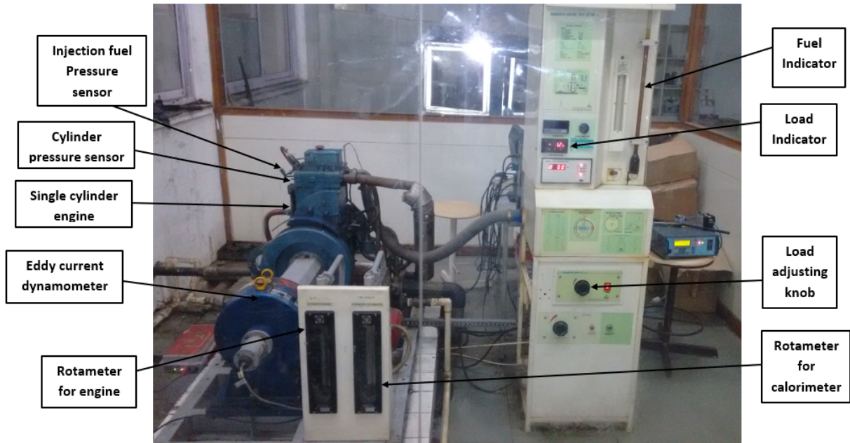
Figure 3.2: Actual experimental engine setup available at the institute
