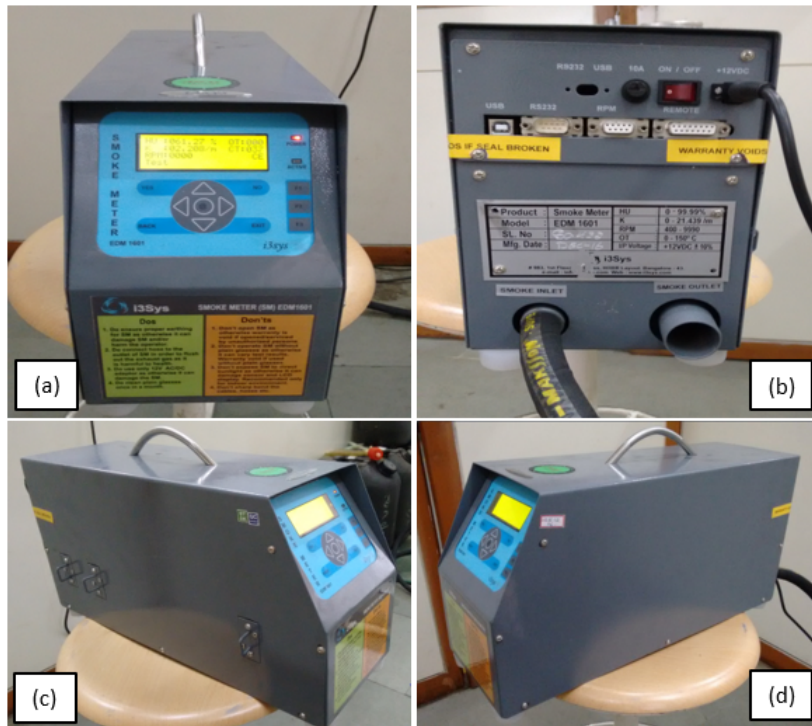
Figure 3.4: Different views of smoke meter (a) Front portion (b) Rear portion (c) Right hand side portion (d) Left hand side portion
