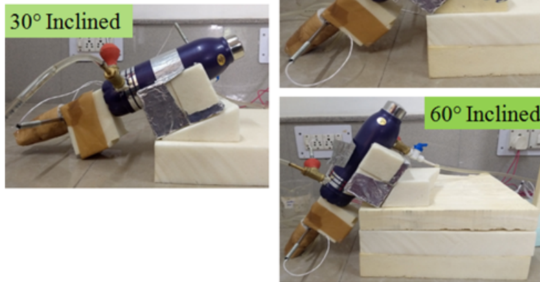
Figure 3.2: Experimental setup of screen meshed heat pipe at different angles of orientation
