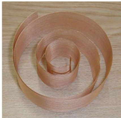
Figure 2.6: Screen Mesh as used for wick inside Heat Pipes [3]
