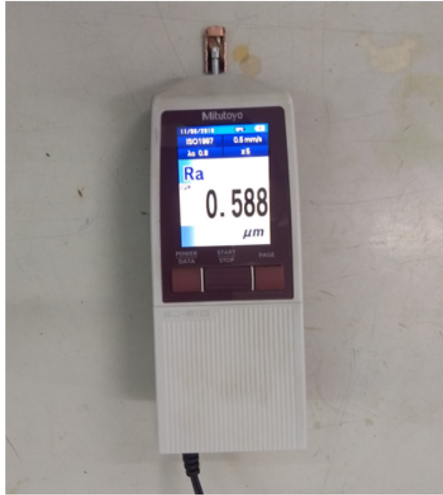
Figure 4.22: Measurement of surface roughness of heat pipe
