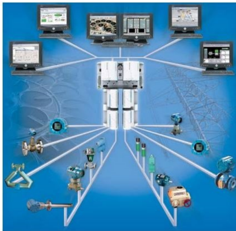
Figure 1.7: operation of DCS
