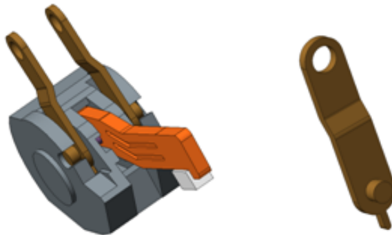
Figure 5.6: Proposed design of drive shaft and drive shaft link
