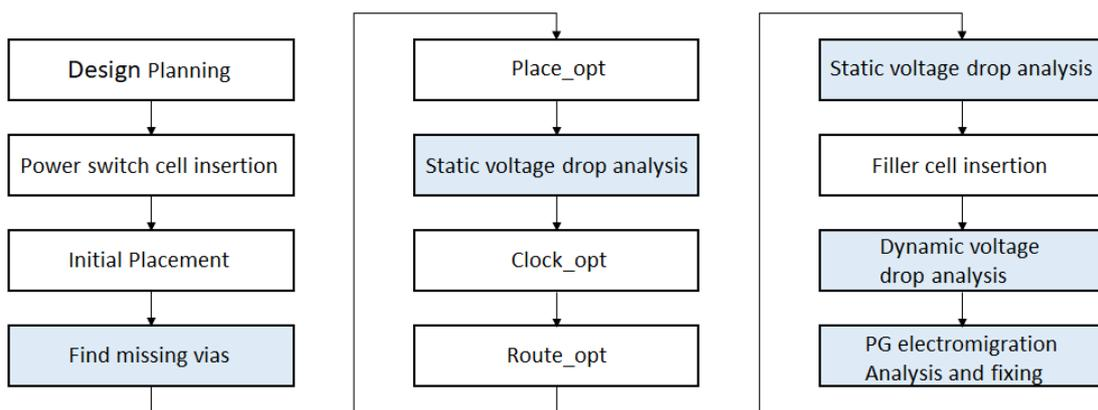
Figure 4.1: Using Redhawk Analysis Fusion in IC Compiler II design flow
