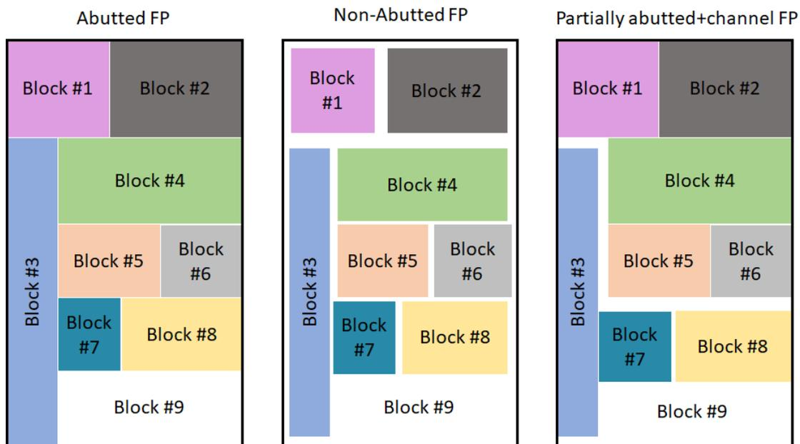
Figure 2.2: Floor plan Techniques
