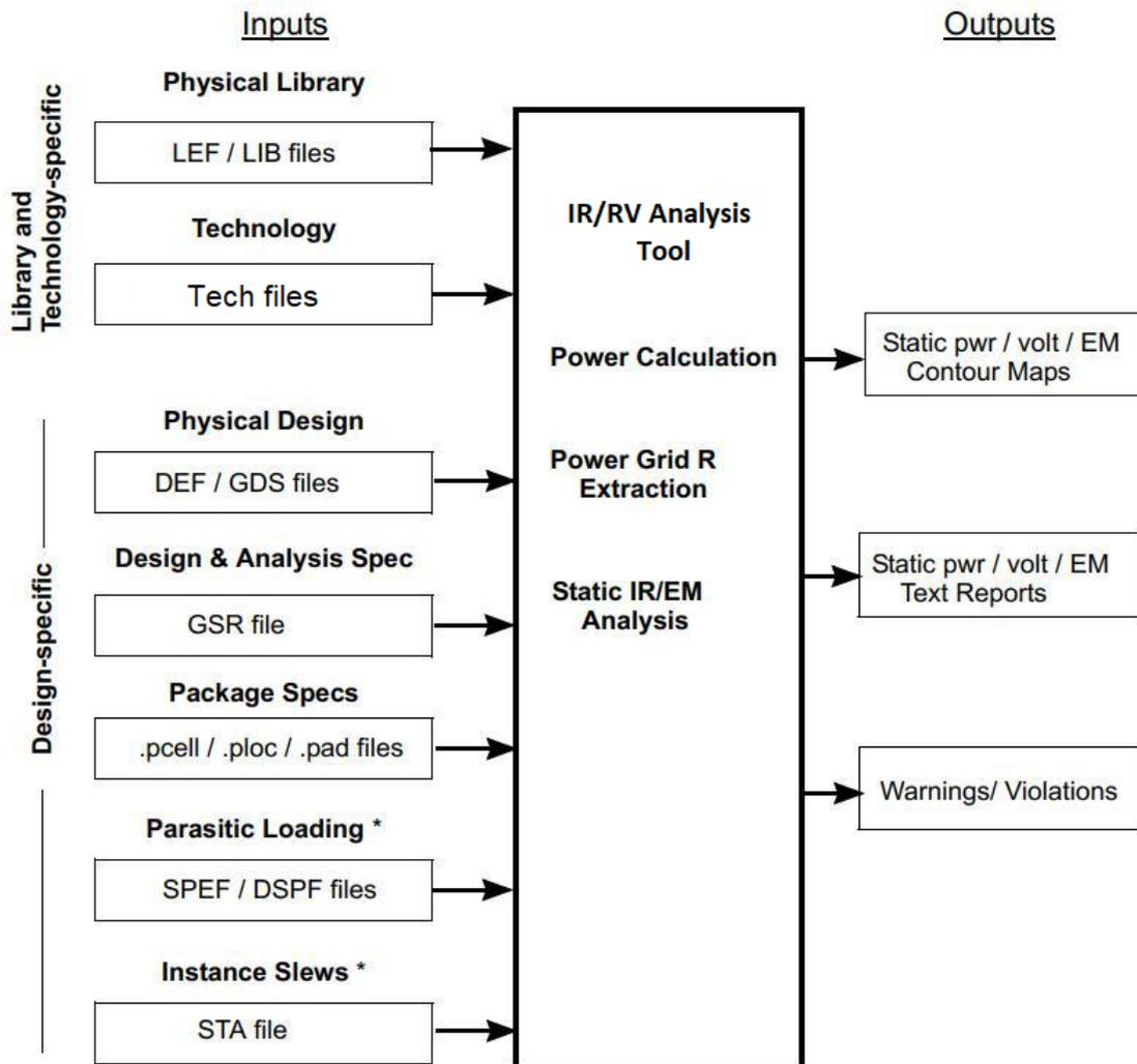
Figure 3.3: Inputs and Outputs of IR/RV analysis tool
