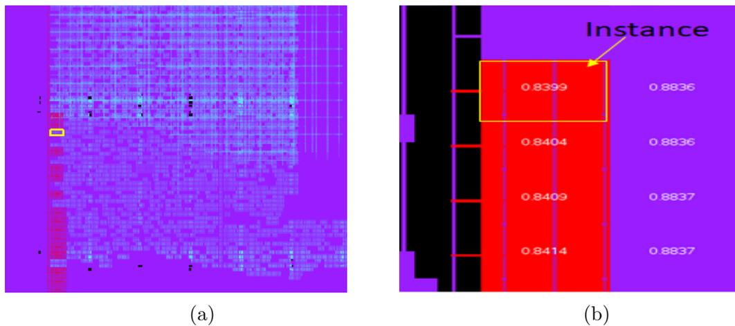
Figure 5.4: (a) Static IR Drop in design, (b) Cells having Static IR Drop violation
