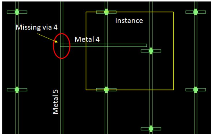
Figure 5.5: Missing via4 of instance having max voltage drop
