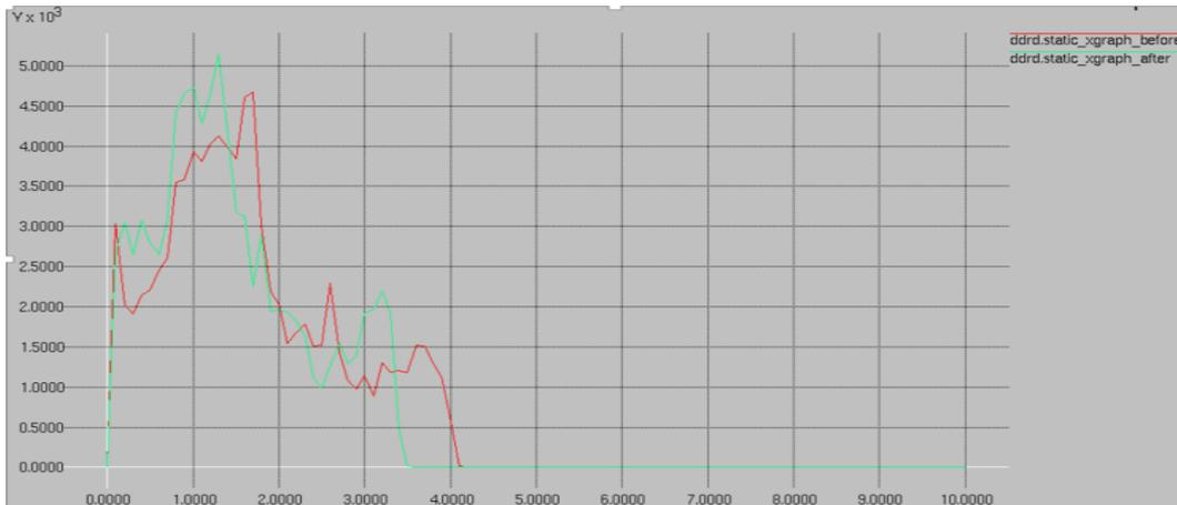
Figure 5.27: Graph of static IR violation with and without IR aware routing
