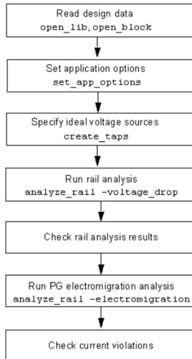
Figure 4.3: Required steps for a basic rail analysis using Redhawk Analysis Fusion
