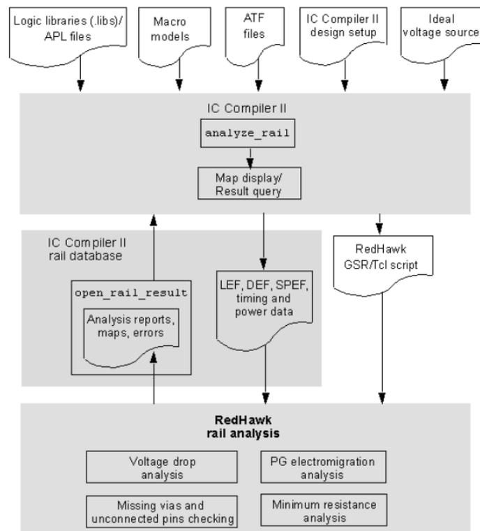
Figure 4.2: Redhawk Analysis Fusion data flow
