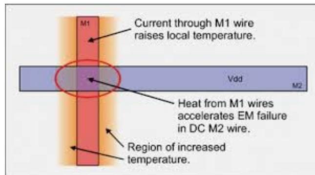
Figure 3.2: Self heating in metal wire
