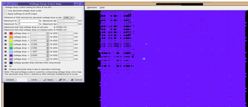
Figure 5.8: Design after cleaning Static IR violation
