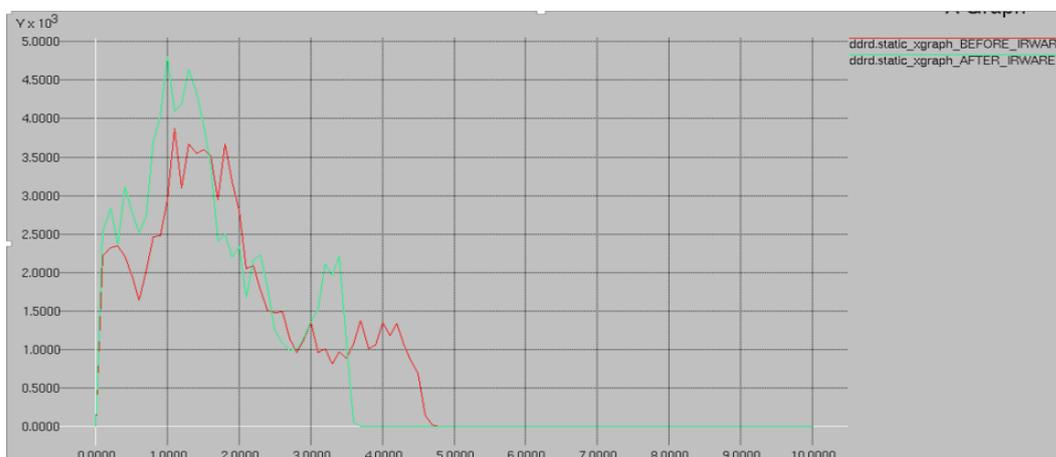
Figure 5.24: Graph of static IR violation with and without IR aware placement
