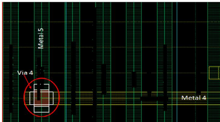
Figure 5.6: Placed via4 between metal4 and metal5 in PNR tool
