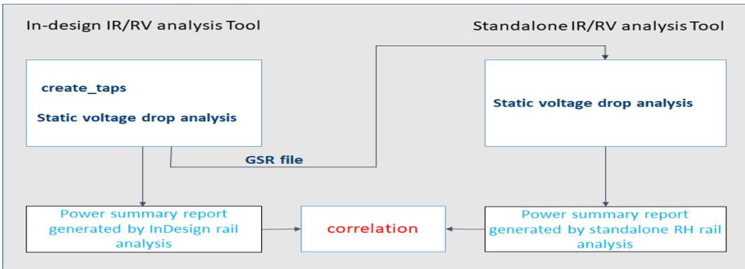
Figure 5.12: Data Flow for static analysis correlation of in-design and standalone IR/RV analysis tool
