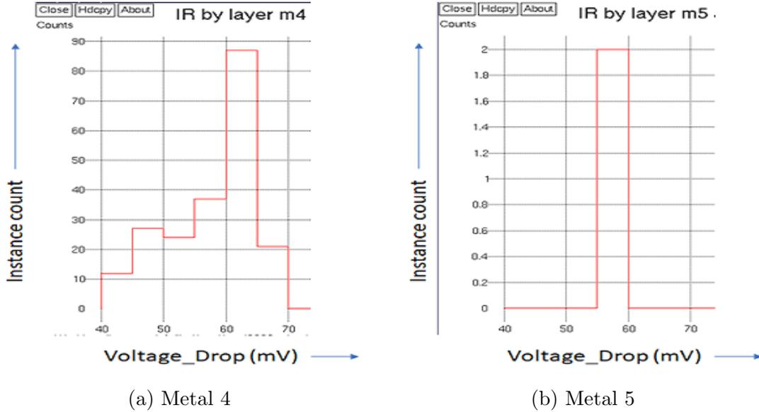
Figure 5.2: Histograms of instances having drop beyond 44.5mV on metal 4 and 5 respectively
