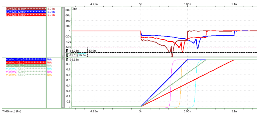
Figure 5.10.2: Leakage in Dual Rail (LS)
