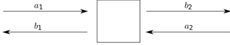
Figure 3.5: Block diagram for representing the S-parameter matrix [13]
