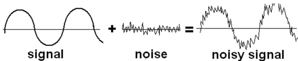
Figure 3.10: Output of a 2-port noisy device [14]
