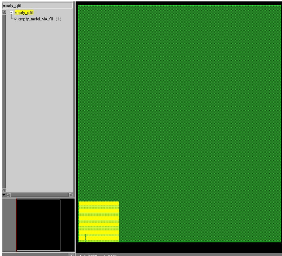
Figure 4.1: Rectangular metal fill done using bbox command
