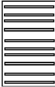
Figure 3.4: End-to-end metal tracks in the input layout design
