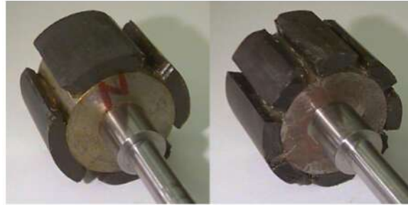
Figure 1.5: 4 Poles and 8 pole-permanent rotor magnet
