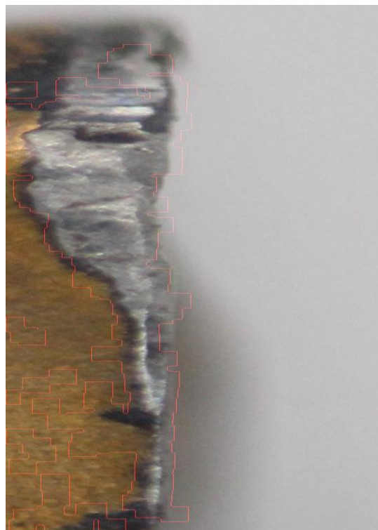
Fig. 28: Identified maximum flank wear region in the tool
