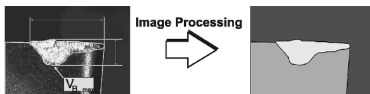
Fig. 9: Image illumination to detect flank wear [4]
