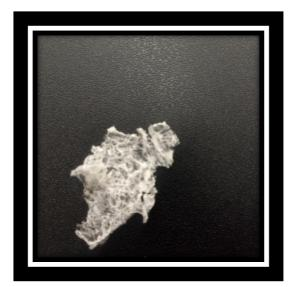
Fig 7: formulated wafers after lyophilization
