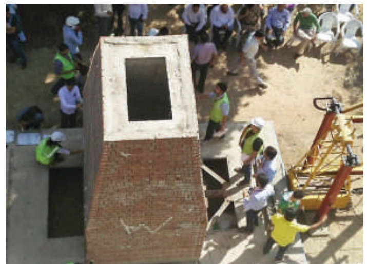
Dynamic Testing of Gopuram Structure through Shock Table Facility
